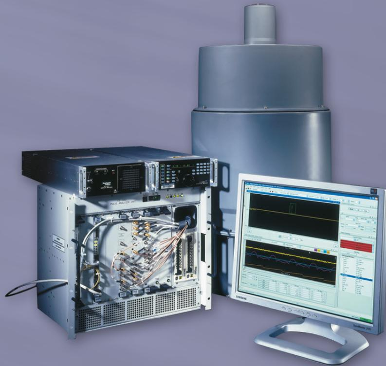
The CS-3030 ELINT/ESM subsystem includes omni and spinning DF antennas, microwave receivers, a radar pulse analyzer and an operator workstation.
